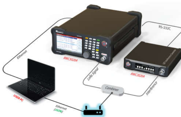
Fig 3.29 CW Interferer test environment
